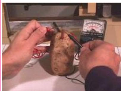
We repeated this experiment with some other fruits and all resulted almost the same. In all cases the produced voltage is between 1 and 1.5 volts, and in all cases they do not produce enough current to turn on a small light.
