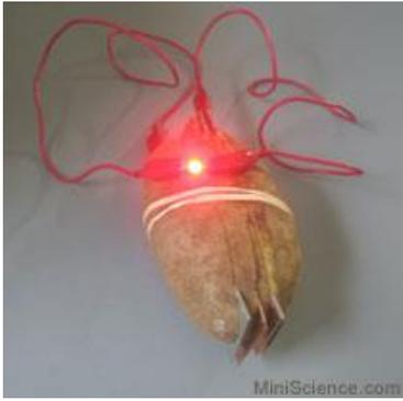
By connecting multiple potato batteries you can make enough electricity to light-up a super bright light emitting diode
